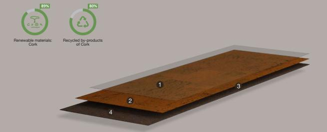
1 AQUADUR waterbased matt finish with CleanSurface technology 2 Natural cork decorative veneer 3 Bevelled edges 4 Expanded black agglomerated cork backing
